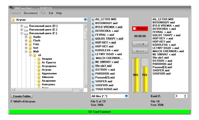
2AVCom Host Software is intended for interfacing between the UniFlash device and a PC. It helps to manage databanks in the musical instrument directly from a PC: copy, delete, change name, format, etc.
